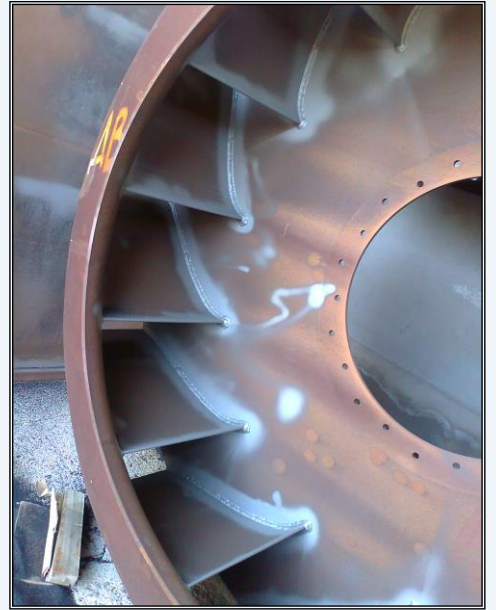
Protect welds seams of smoke extraction turbine from sulfide-oxide corrosion. Coating is NiCrBSi. Bulgaria.
