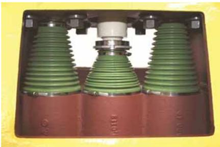
The standard bellows seals are manufactured from Viton but they are also available in H-NBR and in PTFE for special applications.
