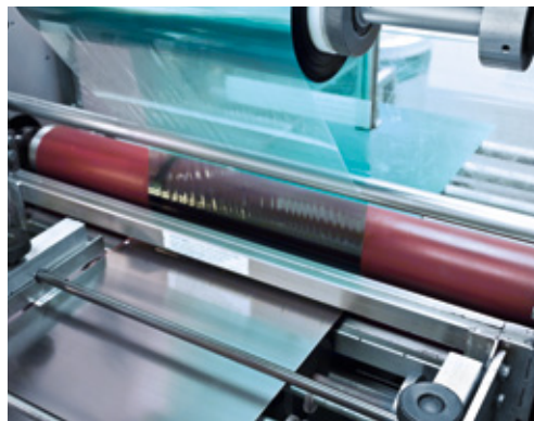
Laminating resistor substrates in cleanroom
