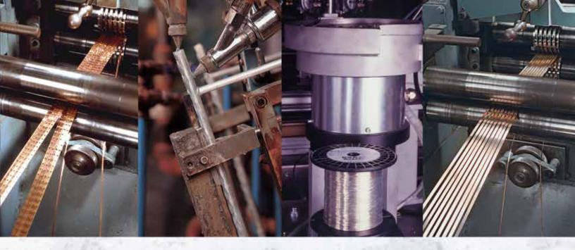
As one example, our flexible wire drawing and flattening process uses carbide and diamond dies to produce wire diameters from .187" to .005" (4.75mm to .127mm).
