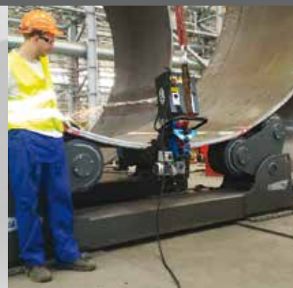
SMUSSO INTERNOTUBO Ø 3000 mm BEVEL ON INTERNAL PIPE dia. 3000 mm
