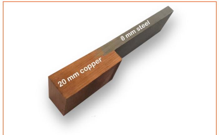
Friction stir welding of dissimilar metals: copper to steel
