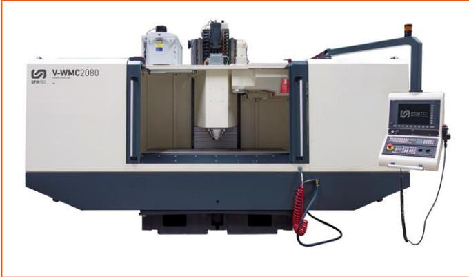
Hybrid FSW CNC machine center V-WMC2080
