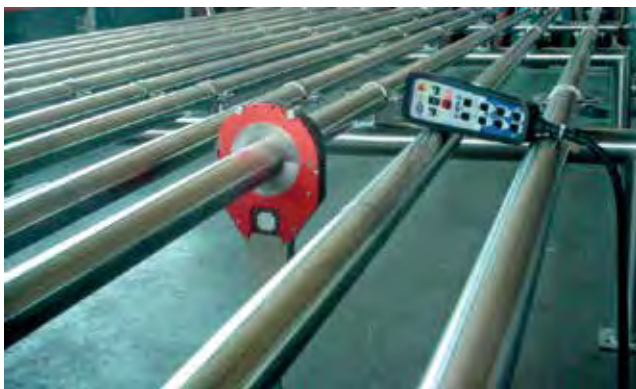
Figure 5. High-quality welding results – work on tubes and fittings is carried out primarily using closed welding heads.
