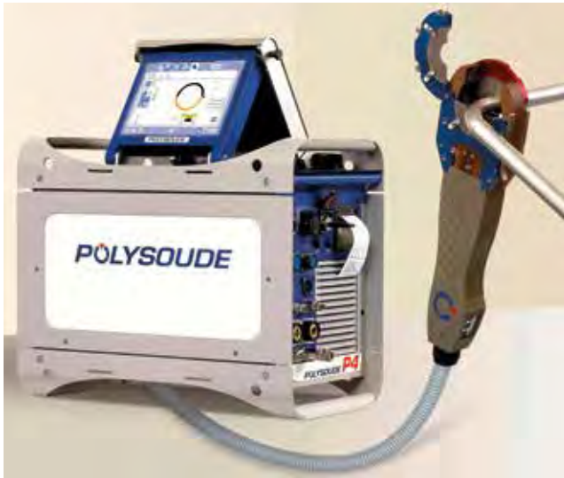
Figure 4. Orbital welding equipment on stainless steel tube.
