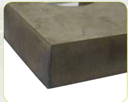
Example of a 20mm cut with WMS
