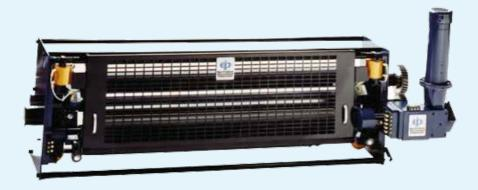
The unique Delta design utilizes helical gears and positive roller settings to drive the dampening form roller at a slower surface speed than the plate cylinder. The differential motion, called the "Delta Effect" wipes away the foreign particles that cause hickeys, while continuously allowing a fresh charge of ink to the plate.
