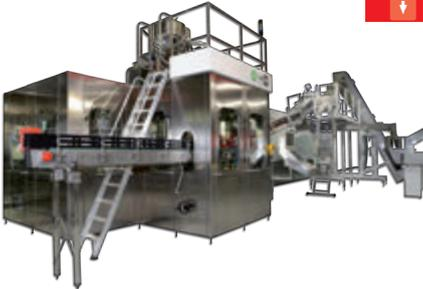
The SBF rotary blow moulding machine can be installed in combination with rotative fillers.
