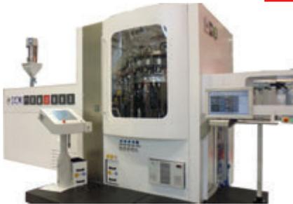
The CBF machine (Compression Blow Forming) is based on a unique, innovative thermoplastic material conversion process that allows producers to obtain a container directly from the granulated material.
