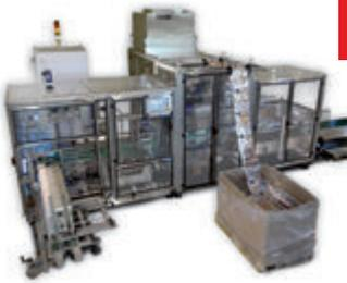
Sacmi Packaging also produces MONOBIB, the replenishment, packaging monoblock that unites all the functions to create Bag in Box type packs. It is made up of the box creator with a hot melt closing, the pouch filler that also includes box insertion and the hot melt box close.
