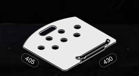
Toe plate to hook on 430 x 405 mm
