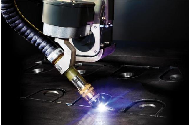
**DMX** This is ESAB's reliable and accurate plasma bevel system. The DMX is not only easy to use but easy to maintain thanks to ESAB's exclusive Direct Multi-Axis motion system and Multi-Point Collision Protection. These mean that the DMX requires fewer parts and automatically resets after a collision, without the need for routine alignments. This affordable and compact machine effectively
