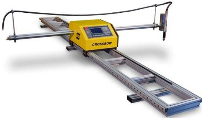
**Crossbow** This machine is lightweight enough for easy transport making it ideal for use in repair shops, trade schools and for portable use in large facilities and construction sites. The Crossbow's precision guide rail facilitates the stable motion of the crossbeam and full support of the cutting torch
