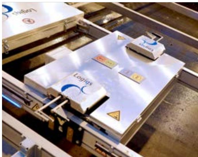
In order to be able to move between rows, the 2D-Shuttle makes use of a X-Rail which usually spans the whole length of the growing area.
