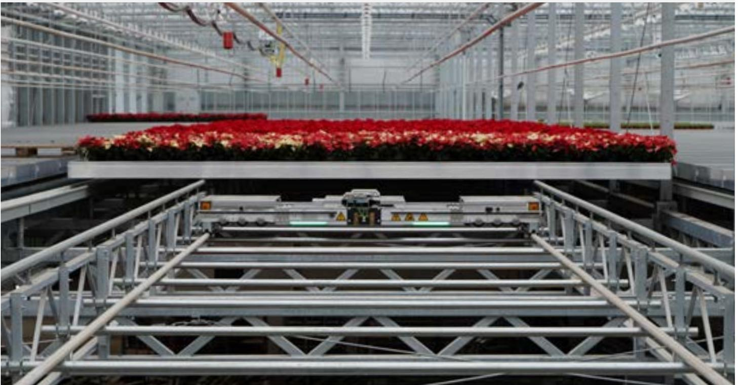
The 2D-Shuttle can also switch rows independent of other machines.
